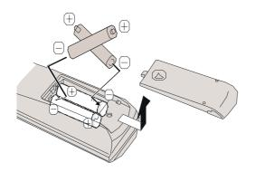
**NOTE:** Remove the batteries from remote control handset when it is not to be used for a long period. Otherwise it can be damaged due to any leakage of battery.
