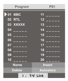
Program Menu is used to delete a channel, to change the programme number of a channel, to give a channel name to a channel, and to start the A.P.S (Autostore) function.
