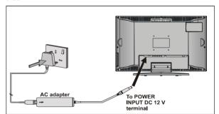
IMPORTANT: The TV set is designed to operate on 12 V DC. For this, an adaptor is used which gives 12V DC voltage. Connect this adaptor to a system that supplies 100 -240V AC, 50/60 Hz.
