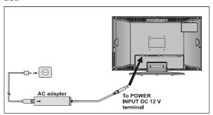
IMPORTANT: The TV set is designed to operate on 12 V DC. For this, an adaptor is used which gives 12V DC voltage. Connect this adaptor to a system that supplies 100 -240V AC, 50/60 Hz.
